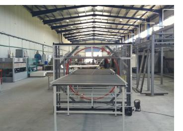
Ease and safety feeding and taking out of film roll. Machine is under sfety mod when chancing the films. Automatic pneumatic control of cutting film and automatic start. Speed of ring is adjustable by inverters. 1Speed of conveyor is adjustable. Object outer packing diameter: **400-400mm**. **700x700mm 900x900mm**.
